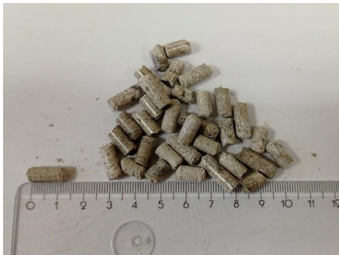
Fig. 2. Main view of produced cylindrical bone and horn meal (BHM) granules
